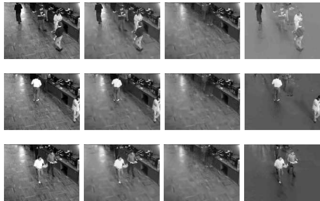
Figure 2: First column: original Restaurant video frames at t = 70, 116, 140 . Second column: frame recovered by NLDR with 30% measurements. Next 2 columns: background and object estimated by rLSDR .
